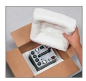
**Step 3:** A top cushion is formed by placing a second Instapak® foam-filled bag on top of the product and closing the carton.
