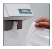
**Step 1:** Press any one of the 10 preset foam amount keys to dispense a foam-filled bag. Remove the bag of expanding foam by tearing at perforations.
