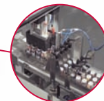
Heavy-duty servo pick and place unit capable of 40 lb. payload
