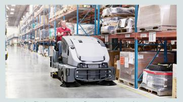
SmartFlow<sup>™</sup> adjusts solution flow with the machine's speed, using water and chemicals. Proportionally higher productivity with fewer dump and refill cycles per tankful.
