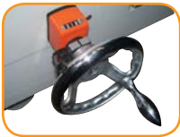
Analog counters simplify changeover
