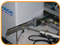
Pneumatic arm squares cases before sealing
