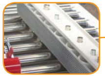
Side belt drive with belt over roller technology
